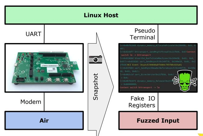
**Emulate Bluetooth firmware** with the same speed as in hardware for realistic **full-stack fuzzing**.
