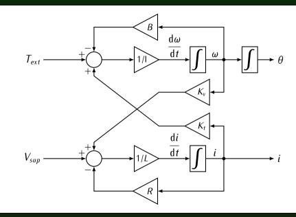
Motor Model Block Diagram
